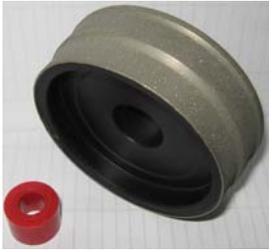
This roughing wheel is designed to be used on glass lenses. The 15mm wide size is an industry standard. Many of our competitor's diamond bond segment are 2mm thick. Ours are 4mm thick for longer life. Ask about our
