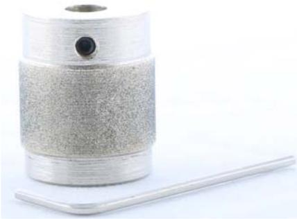
For normal grinding. Fits Glastar's G3, G4, G7, G12, G14, and Inland's Wiz, Wiling, and Wizard Plus. All 4170, 4180, & 4183 bits may be mixed for the quantity price break. Size: 1", 3/4", 1/4", 1/8"
