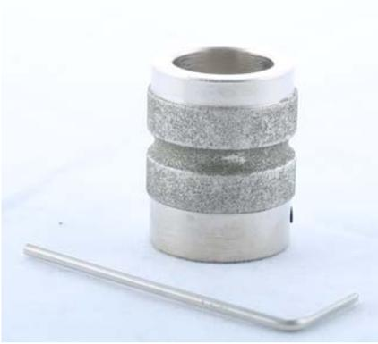
This head has 1 flat and 2 angled surface. Use lower (9 degree) surface for lamps with ten or more panels. To use upper (18 degree) surface for lamps with less than ten panels, lower head on motor shaft, then turn piece of glass upside down to grind correct angle. The flat surface at center may be used for regular flat grinding. Size:
